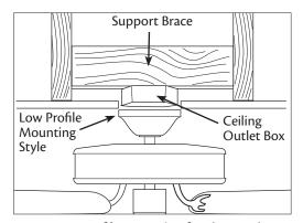
**Low Profile Mounting** fits close to the ceiling, but is not recommended for ceilings less than 8 feet high
